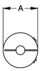
A = 20 D1 = 8 D2 = 8 L = 26 Nom. torque NM (Tkn) = 1.5
